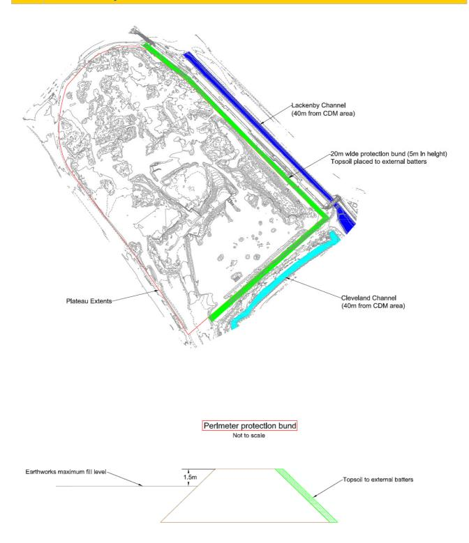
Note: The bund has been constructed so the minimum height of the bund above the maximum fill level when achieved is 1.5m.
